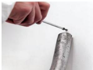
**Figure 7.6** Drilling using a low-speed drill with cowl and fitted with LEV
