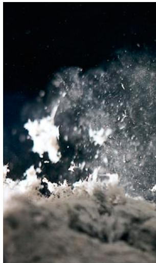
**Figure 1.1** Asbestos fibres being released from lagging
