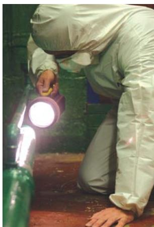
**Figure 7.24** A torch being used to illuminate fine settled dust
